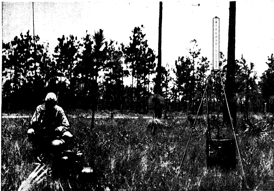
FIG. 20-12.—A moderately good location. The trees are fairly dense, but the sky can still be seen through them. Maximum range will not be greatly reduced.
