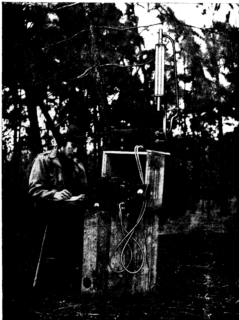
FIG. 20-16.—A poor beacon location. The sky can be seen through the trees in some directions, however. Range will be materially reduced.
